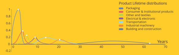
Figure 1: Product lifetime distributions for the eight industrial use sectors plotted as log-normal probability distribution functions  $(\text{PDF})^7$
